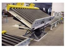
Herkules conveyor lifts simply out last any air or hydraulic lift on the market today. Herkules lifts can be rated for up to a million cycles with a high duty cycle package, by far outlasting similar hydraulic lifts that require maintenance on their electric motors, pumps,
