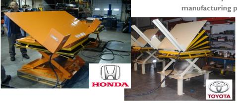
Herkules lift & tilts are only 8" when fully lowered, which allows for increased packing density. The direct lifting air bag all but eliminates load bounce found in competing air lift tables
