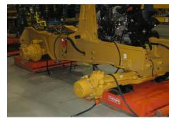
When your application requires the lifting of an extremely heavy load, Herkules has the solution with our direct lifting air bag. Rated for at least 250,000 cycles, and with a low profile of only 6", no other air or hydraulic lift can compete with our VX series lifts. Also inquire about the various built in safety features available.
