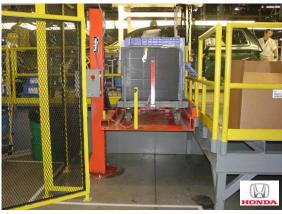
Position the dunnage carts for the associates by lifting, lifting & rotating, tilting, or lifting & tilting the dunnage. Herkules patented direct lifting air bag all but eliminates load bounce and eliminates the need for maintenance that is required
